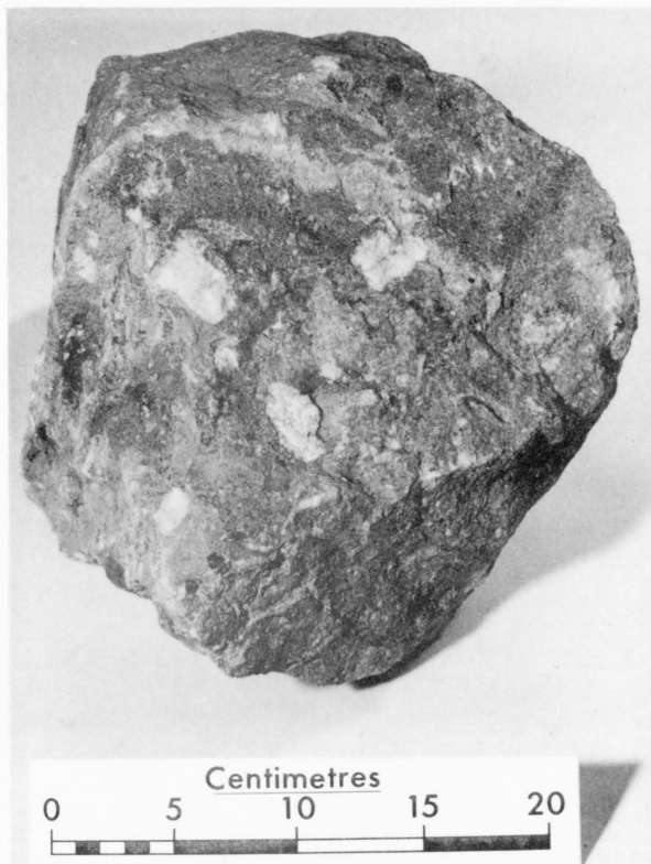
Fig. A. Hand specimen from Dirtlow Rake near Sheldon with angular fragments of calcite set in a fluorite lacking calcite but with minor amounts of barite.
